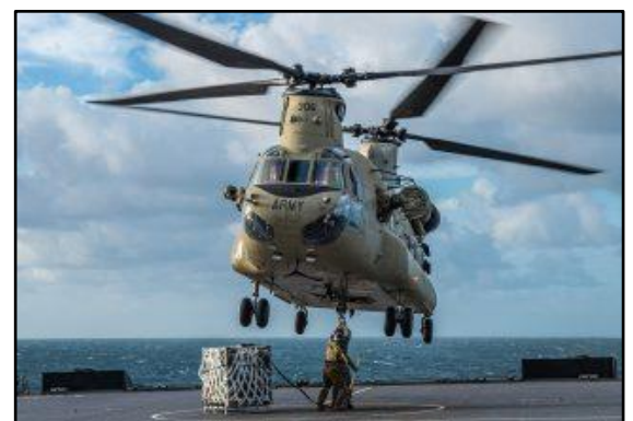
Australian Army CH-47 conducts a class 4 vertrep on the flight deck of HMAS Choules during first of class flight trials in the Coral Sea. Photo: Royal Australian Navy
