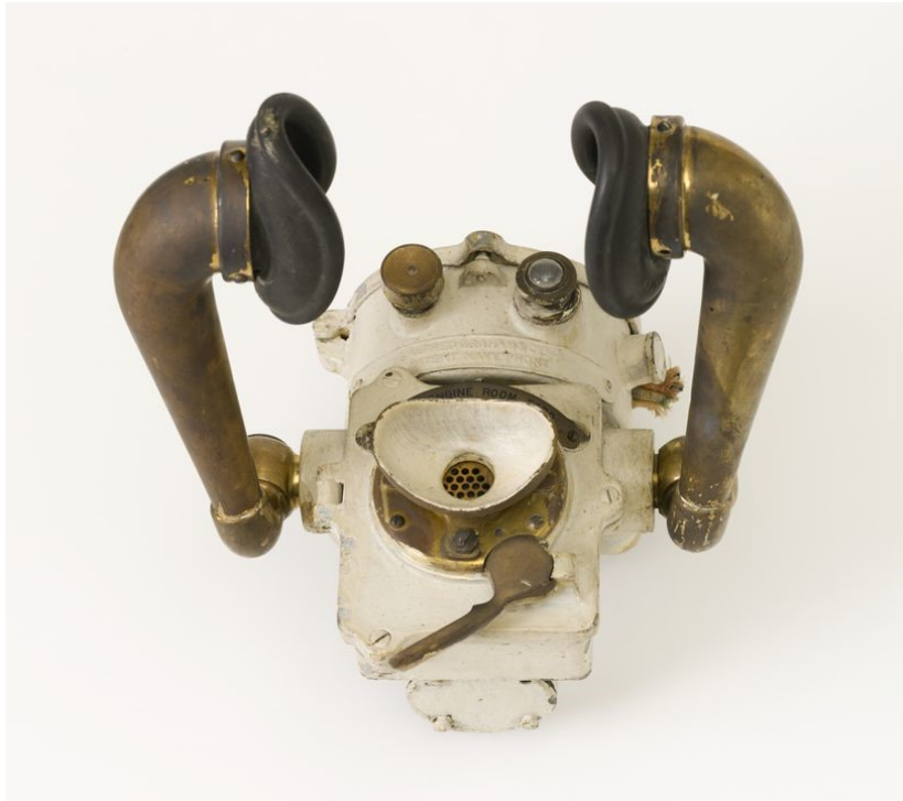
An early naval telephone, made in England by Alfred Graham & Co. in about 1911. It was used on board the battlecruiser HMAS Australia I to communicate between the bridge and the ship's engine room.
