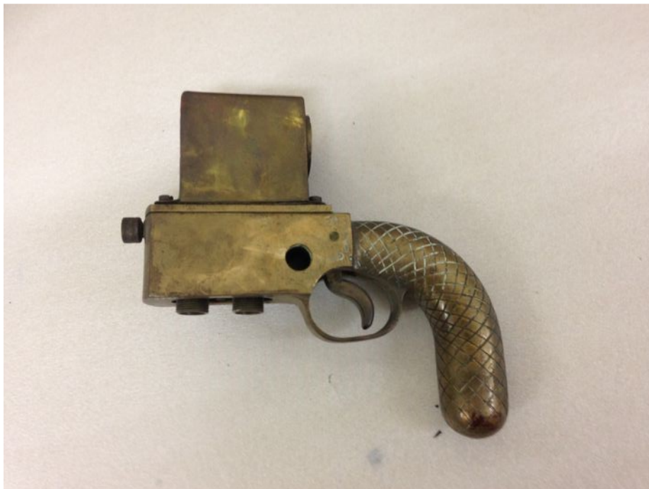
Pistol, electric firing, used on the battlecruiser HMAS Australia. The pistol is a form of contact maker used for local firing of 12 inch gun.
