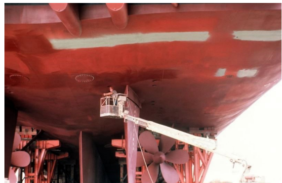
Rudder repairs to USS Wasp (LHD-1). Photo: United States Navy
