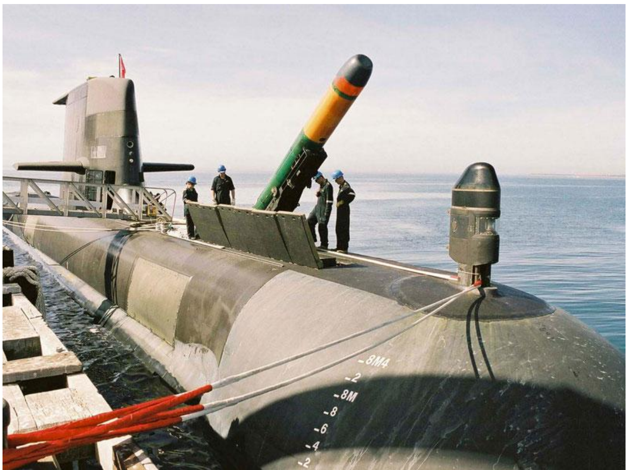
Mk 48 torpedo being embarked into a Collins class submarine. Image courtesy of RAN
