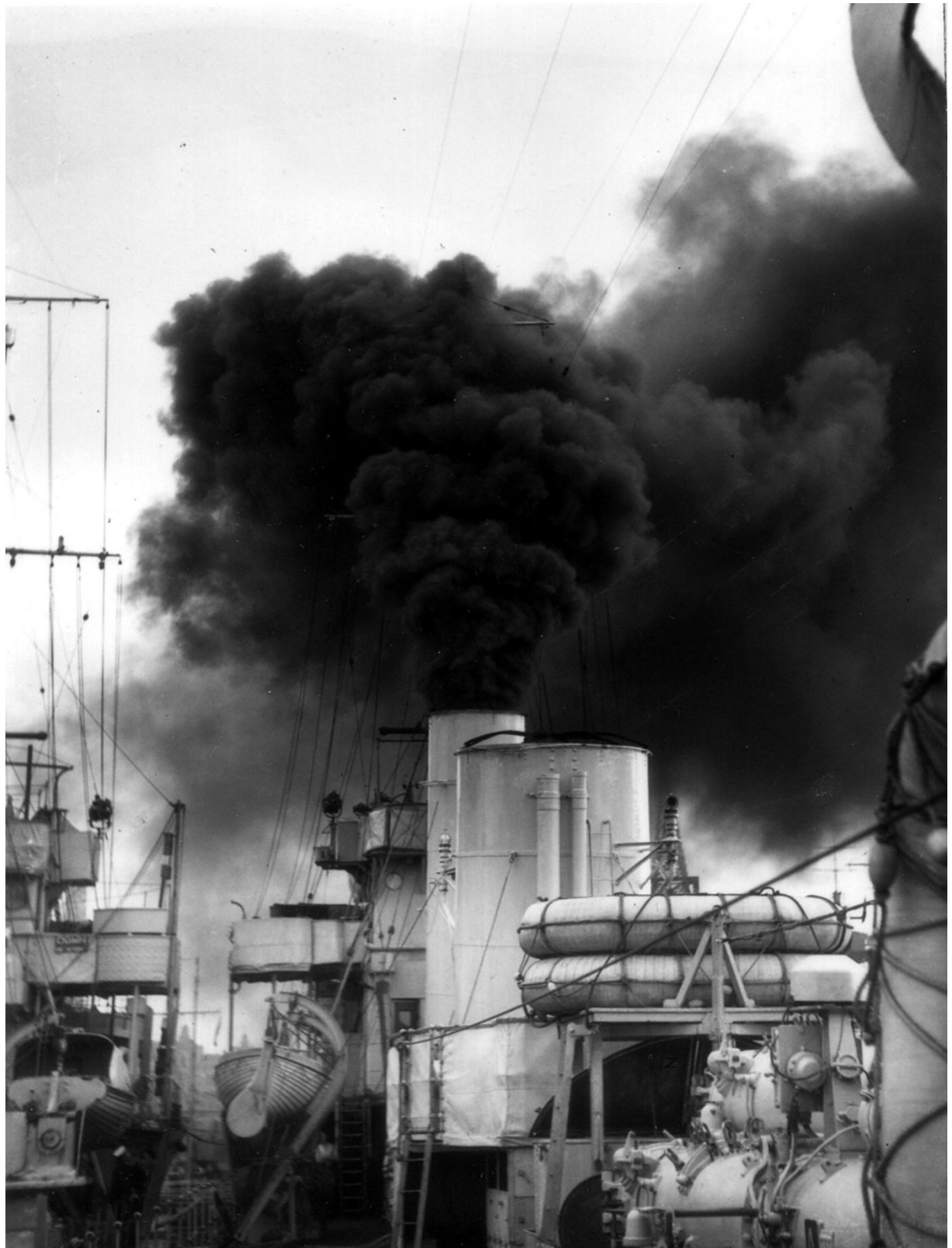
Photo - HMAS Vendetta I - flashing up boilers and getting ready for sea. (Gordon Hill Collection)
