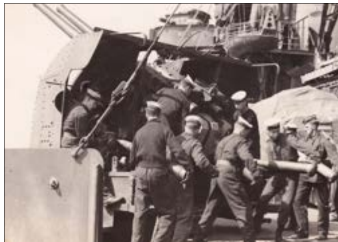
Above: One of the high angle (HA) gun crews loading the MK XVI twin mount. The 35-lb projectile could be fired out to 18,000-yards.
