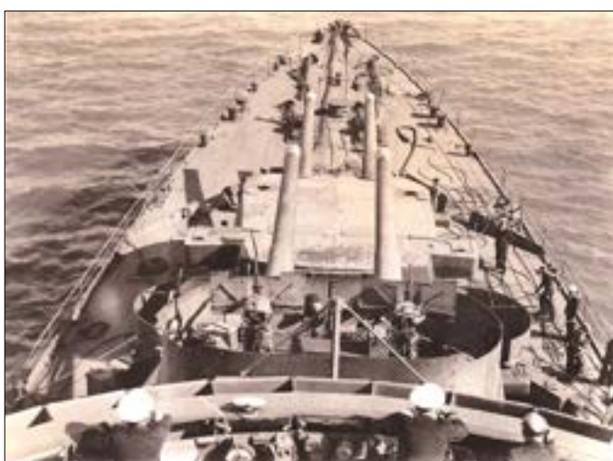
Above: Taken from the foremast, this view looks towards the bow, with the bridge and two forward twin-8-inch gun turrets visible.
