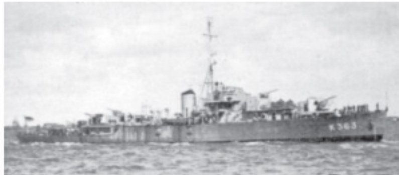
HMAS HAWKESBURY, early 1945. She mounts two 3-barrel "Squid" mortars on the shelter-deck between the two forward guns.
