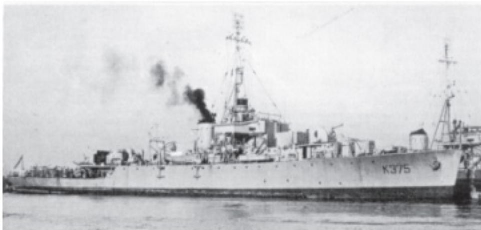
HMAS BARCOO, 1945, before conversion for surveying duties. "Hedgehog" in A position; single 4-in HA/LA on forward shelter deck, another at after end of fo'c'sle deck; 20-mm Oerlikons mounted in bridge wings; surface-warning RDF above the bridge; air-warning RDF on top of foremast.
