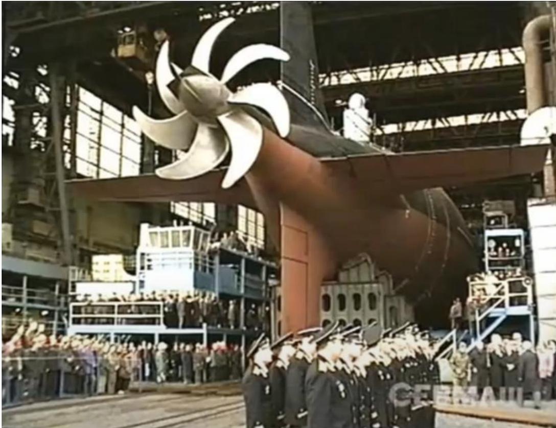
The propeller on an Akula-class Soviet submarine (USN)
