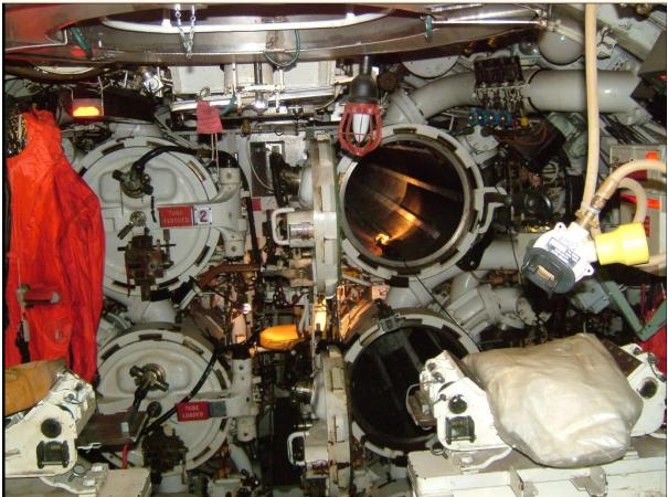
Forward torpedo tubes on the Oberon class HMS Ocelot (RN)
