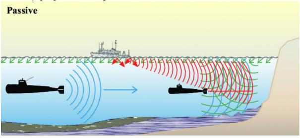
Passive and active SONAR for submarine detection. Passive - the submarine on the right tries to detect sounds (blue) from the other submarine using a towed array (antenna).
