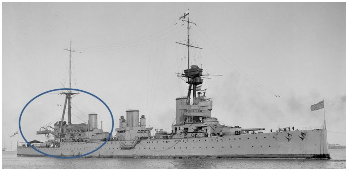
HMAS Australia 1 with ships boats slung on very high davits adjacent the main mast and
