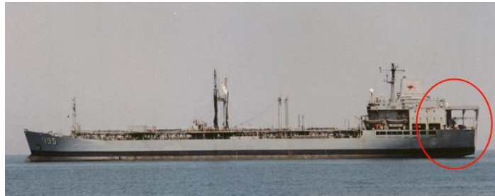
Fast Tracked Configuration changes. Left CIWS fitted to HMAS Brisbane. Above VERTREP deck fitted to HMAS Westralia
