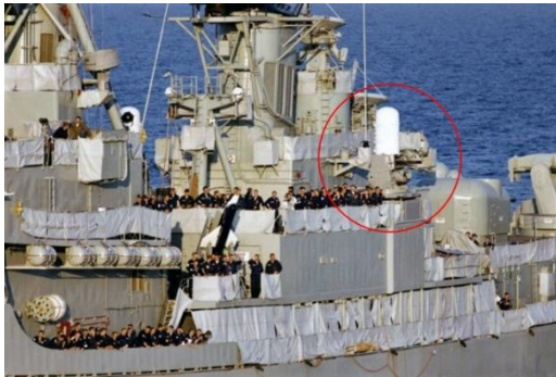
Fast Tracked Configuration changes. Left CIWS fitted to HMAS Brisbane. Above VERTREP deck fitted to HMAS Westralia
